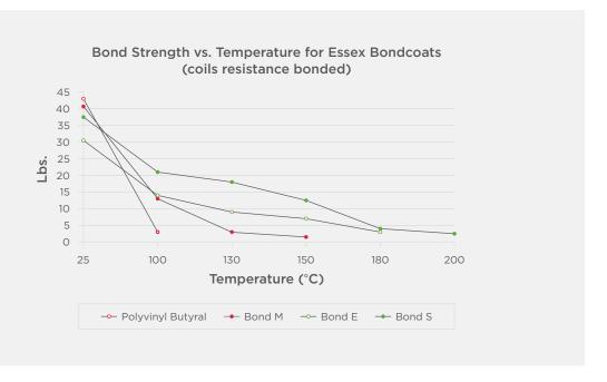
Note: Helical coil bond strength per NEMA MW 1000
