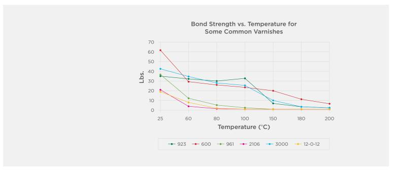
Note: Helical coil bond strength per NEMA MW 1000
